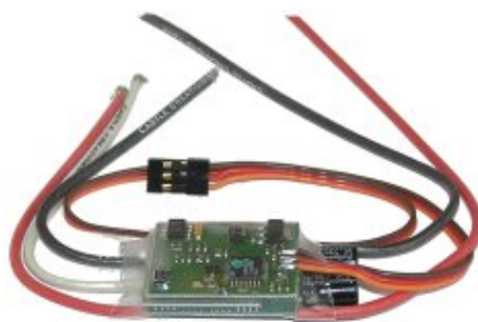
Phoenix 35 ESC showing the BEC side
